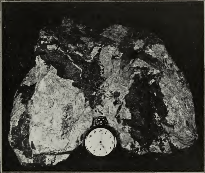
FIG. 5. Rock specimen from dump of Hudson Fluorspar Mine, near Salem, Kentucky, showing remnants of dark gray limestone surrounded by vein calcite. The ragged contacts indicate that the limestone has been partly replaced by the calcite.
